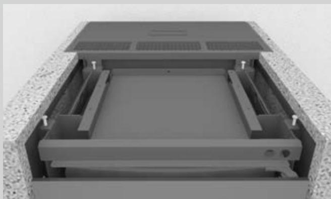
Adjust the top plate screws until there is a 2 cm gap between screw and top edge of stone element.
